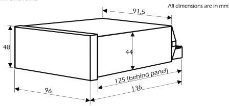
Panel cutout should be 92mm wide x 45mm high, +1mm, -0mm 1/8 DIN. Depth behind panel 125mm max, including cables.
