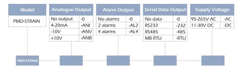
Example - PMD-STRAIN display with 4-20mA output, 2 alarms, RS485 output and 110V AC powered Order code will be: PMD-STRAIN-ANI-AL2-485-AC
